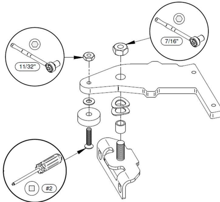
***The nuts must be fully tightened.***
