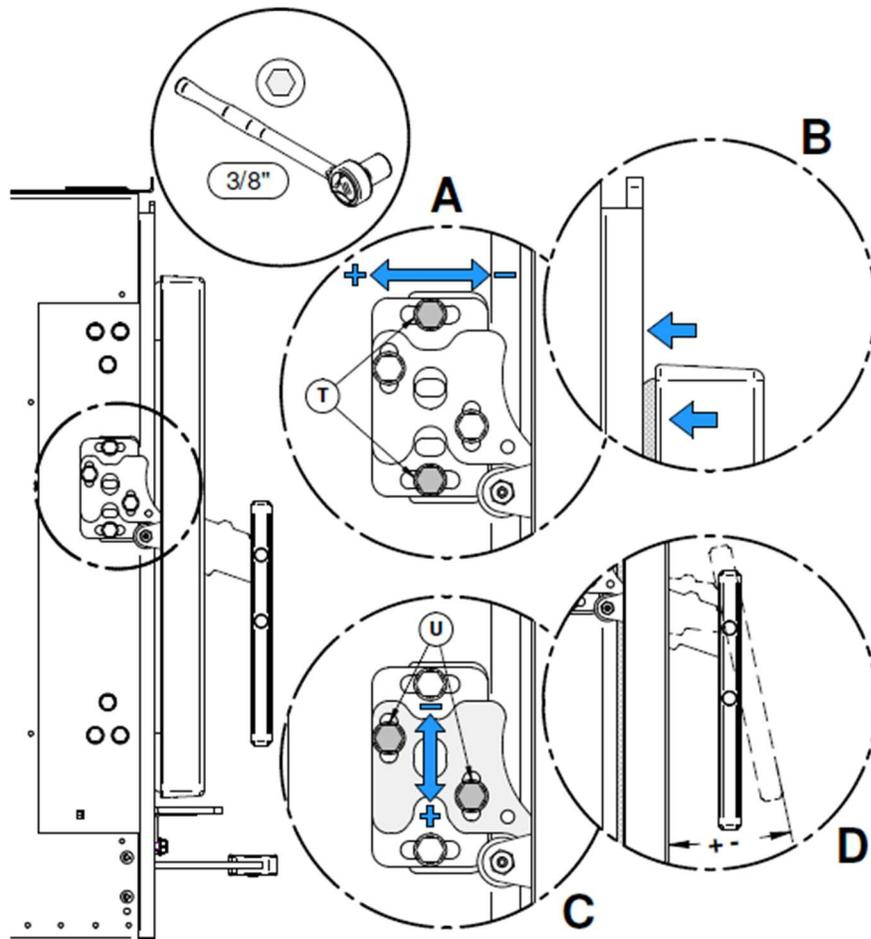
7. **Open the door and squeeze a strip of paper between the door and the combustion chamber. Close the door and pull the paper strip and seek for resistance. Repeat the**
