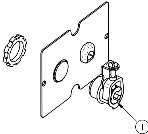
7. Pass the new wires through the connector **(I)** and install the sleeve **(J)** supplied with the manual kit on the BX wire.
