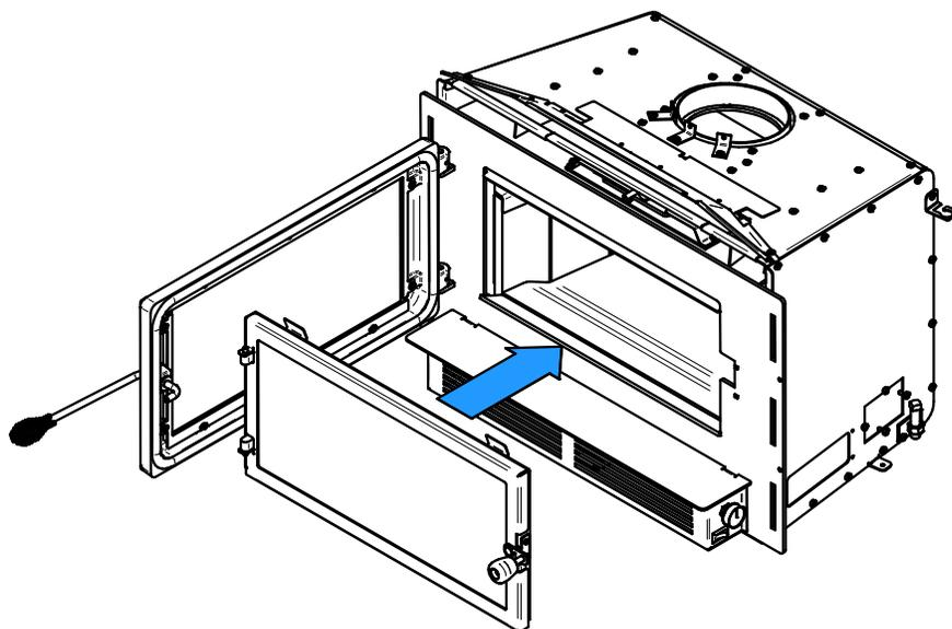
3. Lean the upper part of the fire screen against the top door opening making sure to insert the top fire screen brackets in front of the primary air deflector.
