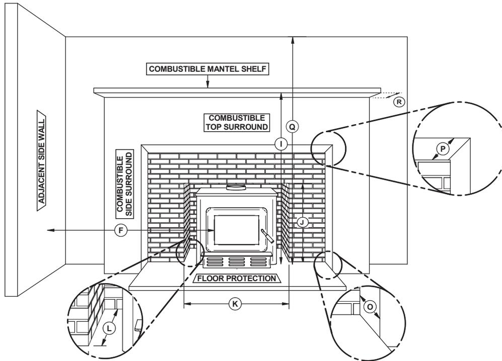
Figure 1 : Hearth opening and clearances to combustibles
