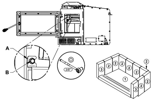
Figure 7 : Remove brick supports
