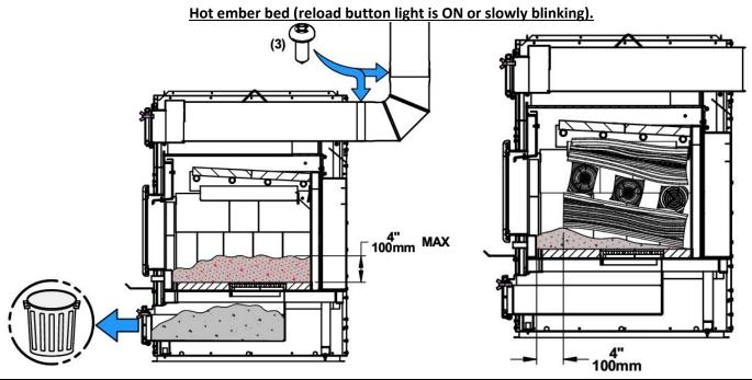
Max 4" of embers and ash accumulation at the bottom of the firebox. If more than 4", increase the target temperature on the thermostat or remove ash when the unit has cooled down. Empty your ash pan every week.
