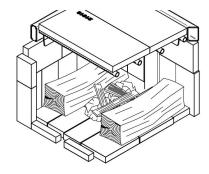
4. Open the door and load your firebox: Place paper and kindling on top of the ash grate, place logs North-South on each side, next crisscross logs on-top of them. LEAVE AIR SPACE BETWEEN LOGS FOR CLEAN AND POWERFUL START!
