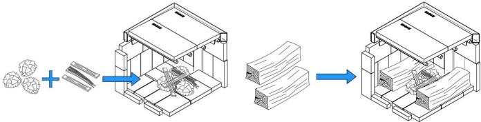
Press the reload button before opening the door. Put paper and kindling on top of the ash grate to help reignite.
