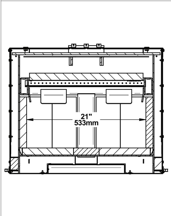
Figure 6 : Front View - Combustion Chamber
