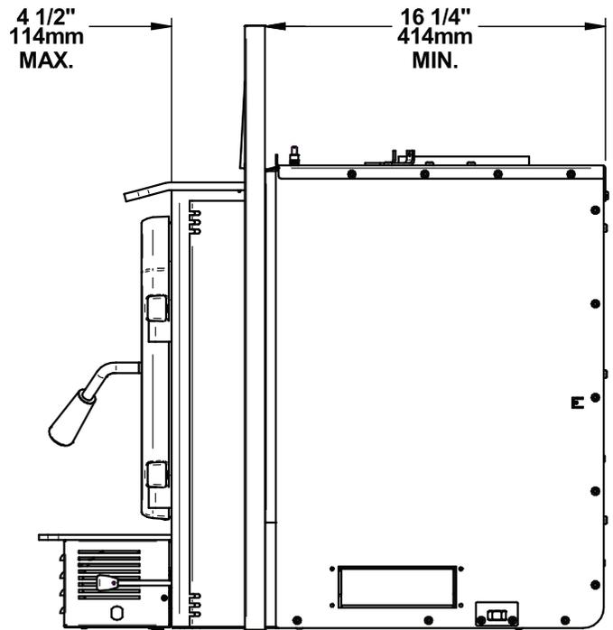
Figure 4 : Side View - Maximum Insert Projection
