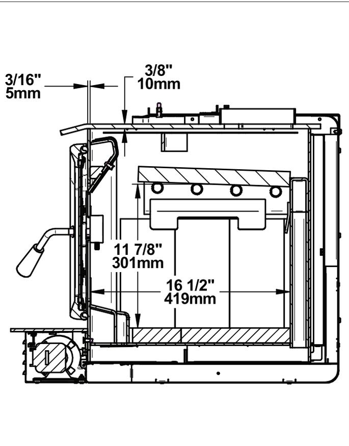
Figure 7 : Side View - Combustion Chamber
