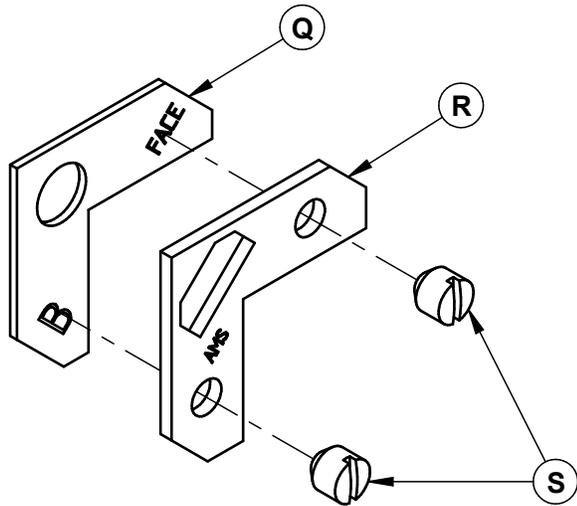
4. Insert the superimposed brackets **(Q)** and **(R)** in the groove of each decorative trim **(T)**, **(U)** and **(V)**. Align the corners of the angled side of each trim, and then tighten the screws **(S)** to secure the trims.
