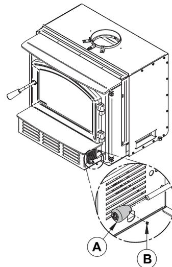
Figure 12 : Installing the air control wood handle
