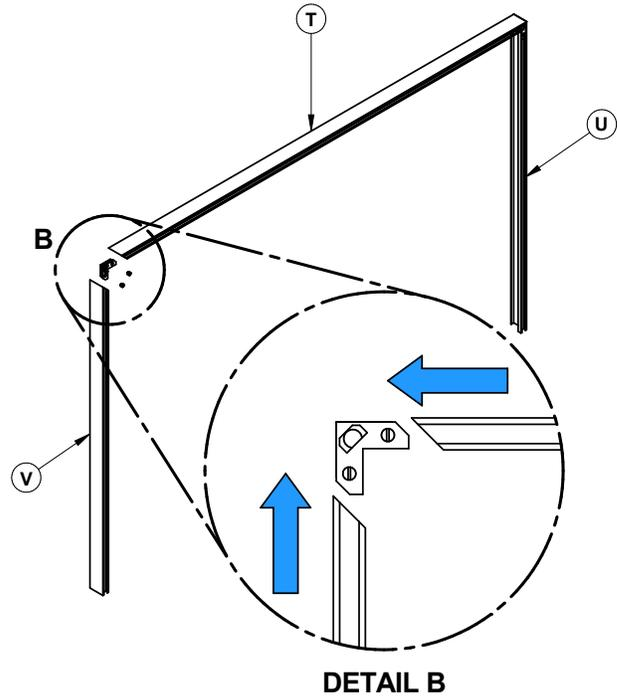
5. Align the trim assembly with the left and right edge of the faceplate and slowly slide it down over the faceplate.
