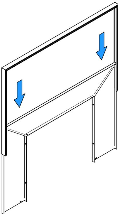
6. Secure the trim to the faceplate by squeezing the eight trim retainers **(W)** between the inner edge of the trim and the front of the faceplate.
