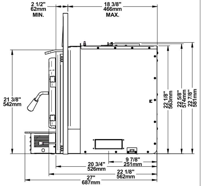
Figure 2 : Side View - Minimum Insert Projection
