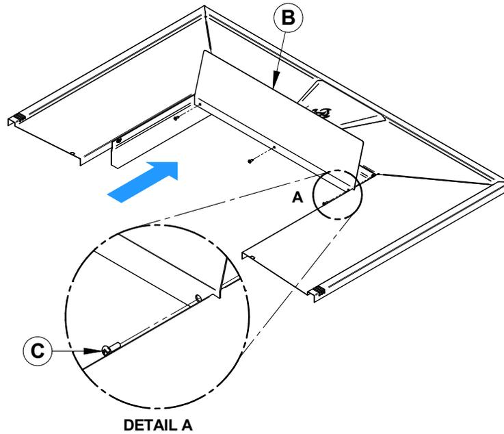
1. Install the heat shield **(B)** on the faceplate (assembled with the faceplate extension) using 3 self-drilling screws **(C)** included in the kit. The heat shield should be pointing upwards.
