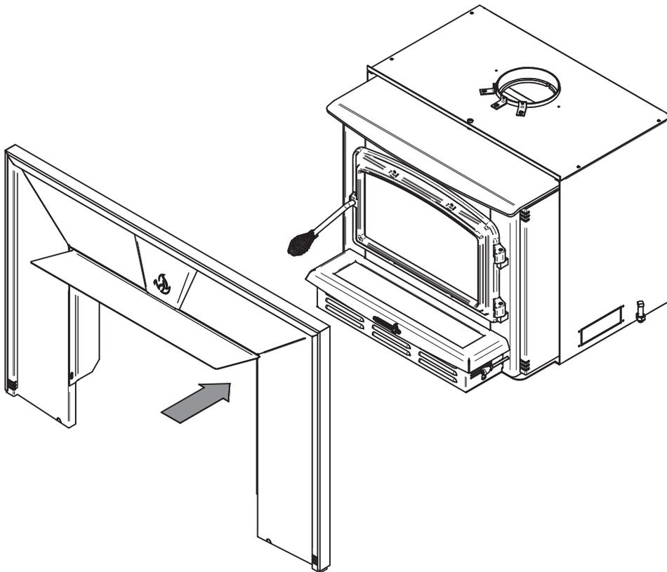
2. Once the heat shield is positioned, install the faceplate on the insert.
