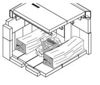
4. Open the door and load your firebox: Place paper and kindling on top of the ash grate, place logs North-South on each side, next crisscross logs on-top of them. LEAVE AIR SPACE BETWEEN LOGS FOR CLEAN AND POWERFUL START!
