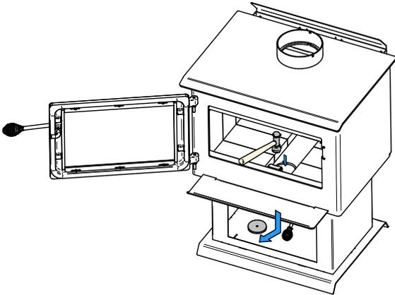
4. Place the ash pan support (A) in the bottom of the base of the stove.
