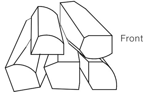
Figure 15: Example low burn load (side view)
