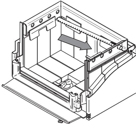
2. Align the notch in the left end of the tube with the key of the left air channel hole. Using a « Vise grip » hold the tube and lock it in place by turning the tube as shown. Make sure the notch reaches the end of the key way.
