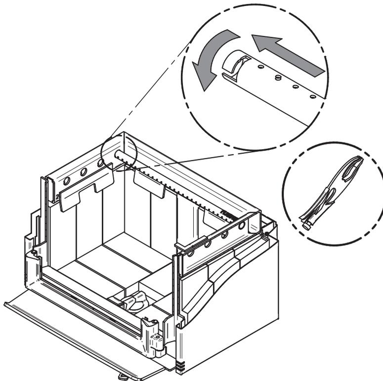
3. Put the baffle in place.
