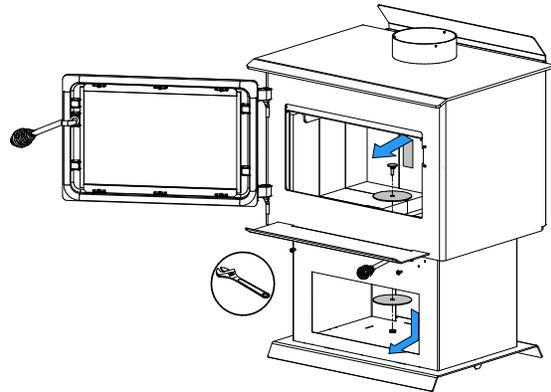
3. Using a hammer, remove the third metal rounds.
