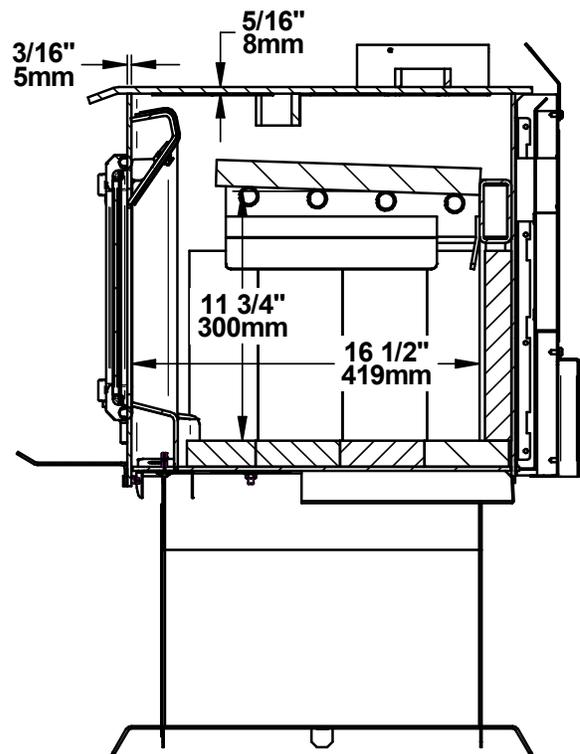
Figure 6: Side View - Combustion Chamber
