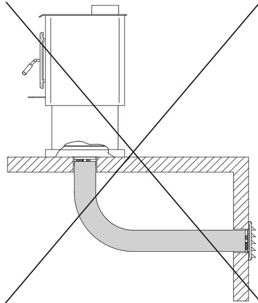
This mobile home approved stove requires the installation of a fresh air intake kit **(A)** and an insulated fresh air intake pipe (HVAC type, must meet ULC S110 or UL 181 class 0 or class 1) **(B)**, sold separately. Refer to air intake kit installation instructions for more details.
