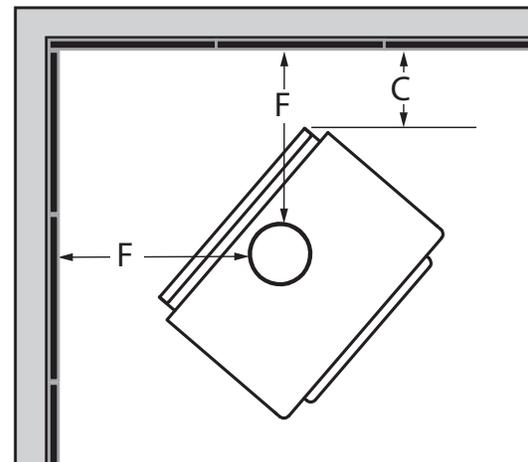
**If the clearance reduction is on the same side as the door handle, position the stove at a minimum of 6 inches from the side wall (clearance B), otherwise it may be located at the clearance shown in the table above.**
