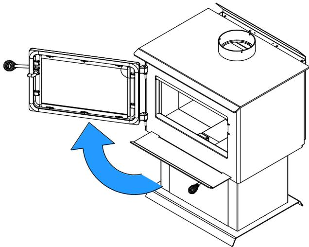
2. Hold the fire screen by the two handles and bring it close to the door opening.
