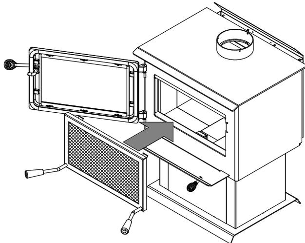
3. Lean the upper part of the fire screen against the top door opening making sure to position the top fire screen brackets behind the primary air deflector.
