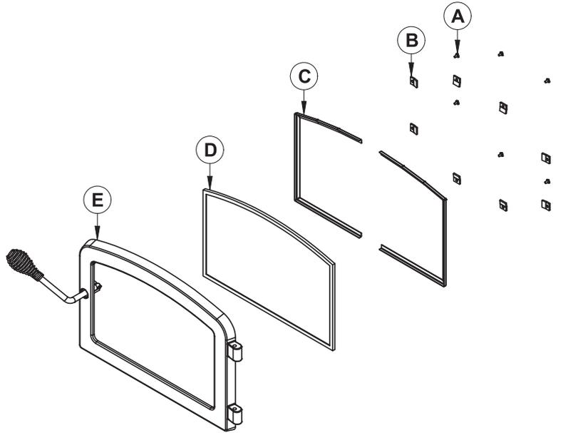
1. Remove the door **(E)** from its hinges and lay it on a soft, flat surface.
