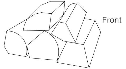
Figure 18: Example medium burn load (side view)
