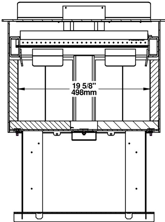
Figure 5: Front View - Combustion Chamber
