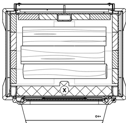
Figure 10: Position of the bottom pieces (High burn)
