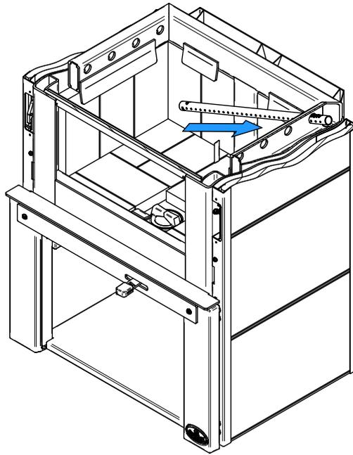
1. Starting with the rear tube, lean and shove the right end of the secondary air tube into the rear right channel hole. Then lift and shove the left end of the tube into the rear left channel.
