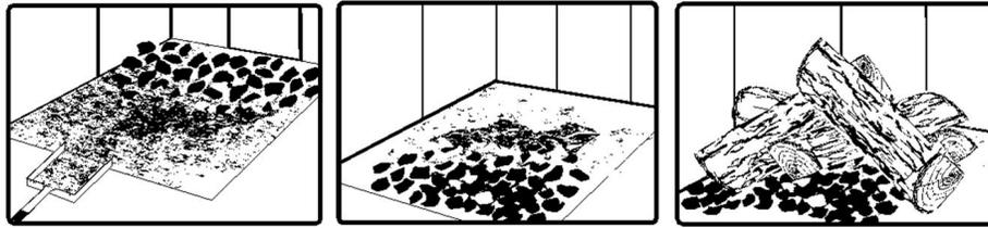
Raking the coals is useful for two reasons. First, it brings them near where most of the combustion air enters the firebox. This will ignite the new load quickly. Secondly, the charcoal will not be smothered by the new load of wood. When the embers are simply spread inside the combustion chamber, the new load smoulder for a long time before igniting.
