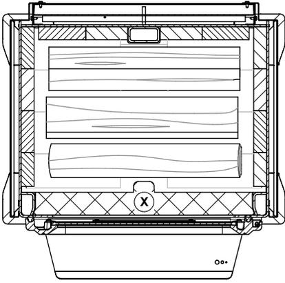
Figure 13: Position of the bottom pieces (Low burn)
