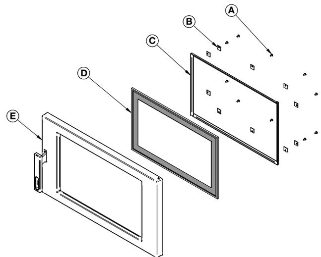
*The two main causes of broken glass door are uneven placement in the door and over-tightening the retaining screws.*
