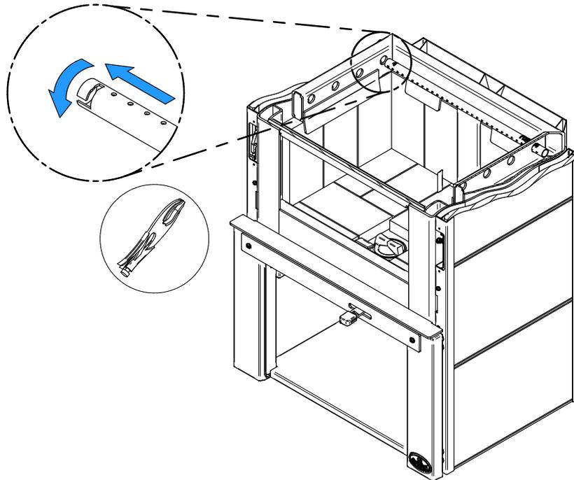
2. Align the notch in the left end of the tube with the key of the left air channel hole. Using a « Wise grip » hold the tube and lock it in place by turning the tube as shown in detail A . Make sure the notch reaches the end of the key way.
