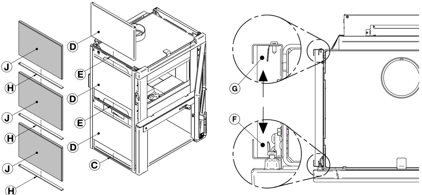
4. Tighten all the screws **(C)** previously unscrewed to hold the decorative assemblies.
