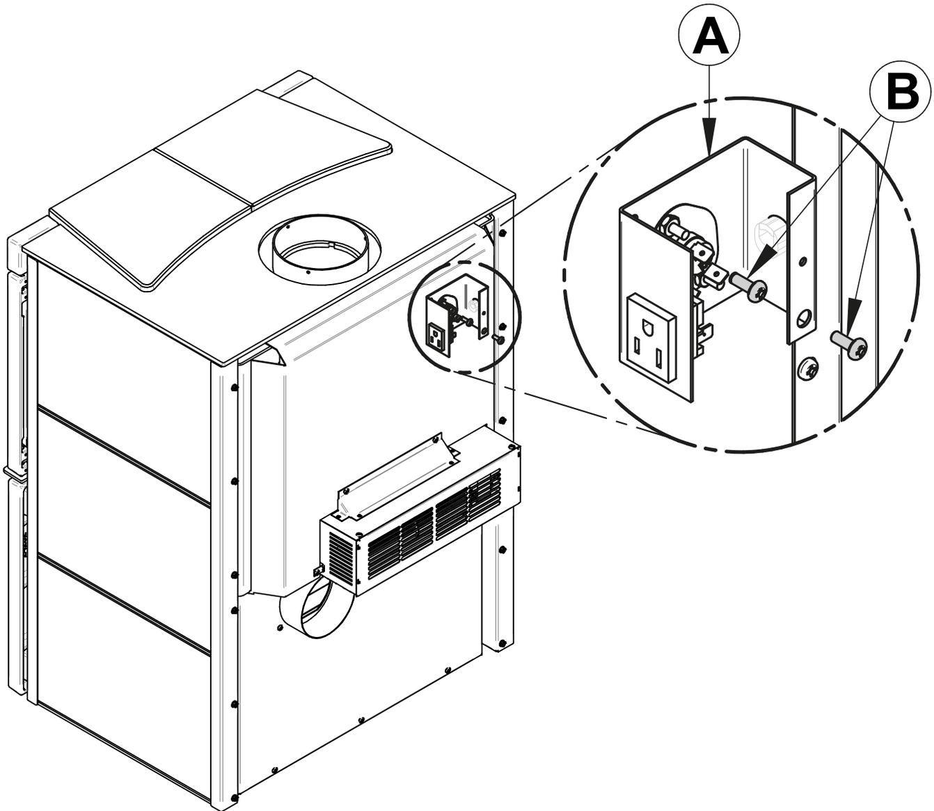
Screw the thermodisc **(A)** on the back of the stove with the screws **(C)** provided.
