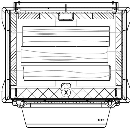
Figure 16: Position of the bottom pieces (Medium burn)
