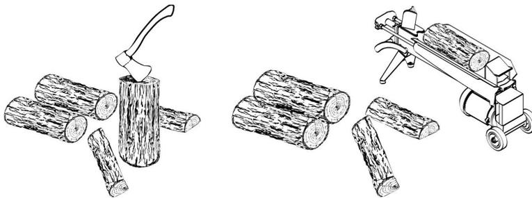
Wood should be split to a range of sizes, from about 3" to 6" (75 mm to 150 mm) in cross section. Having a range of sizes makes starting and rekindling fires much easier.
