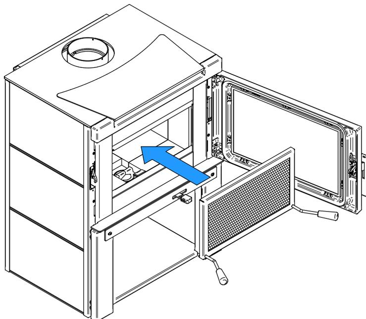
3. Lean the upper part of the fire screen against the top door opening making sure to stove the top fire screen brackets behind the primary air deflector.
