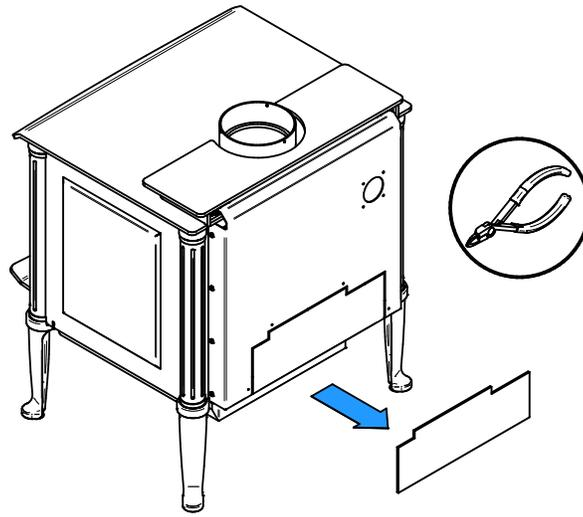
1. Remove the backplate by cutting the knockouts with pliers.
