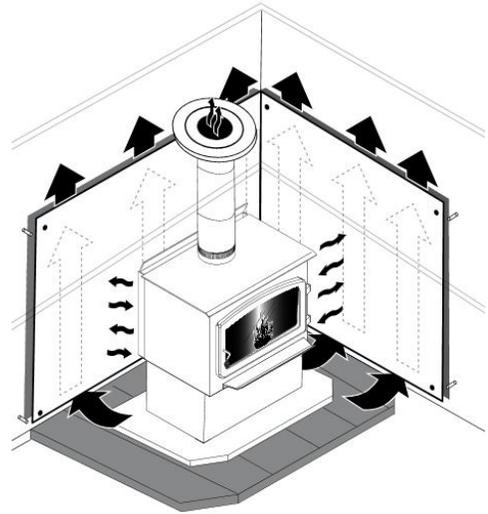
Figure 19: Heat shield
