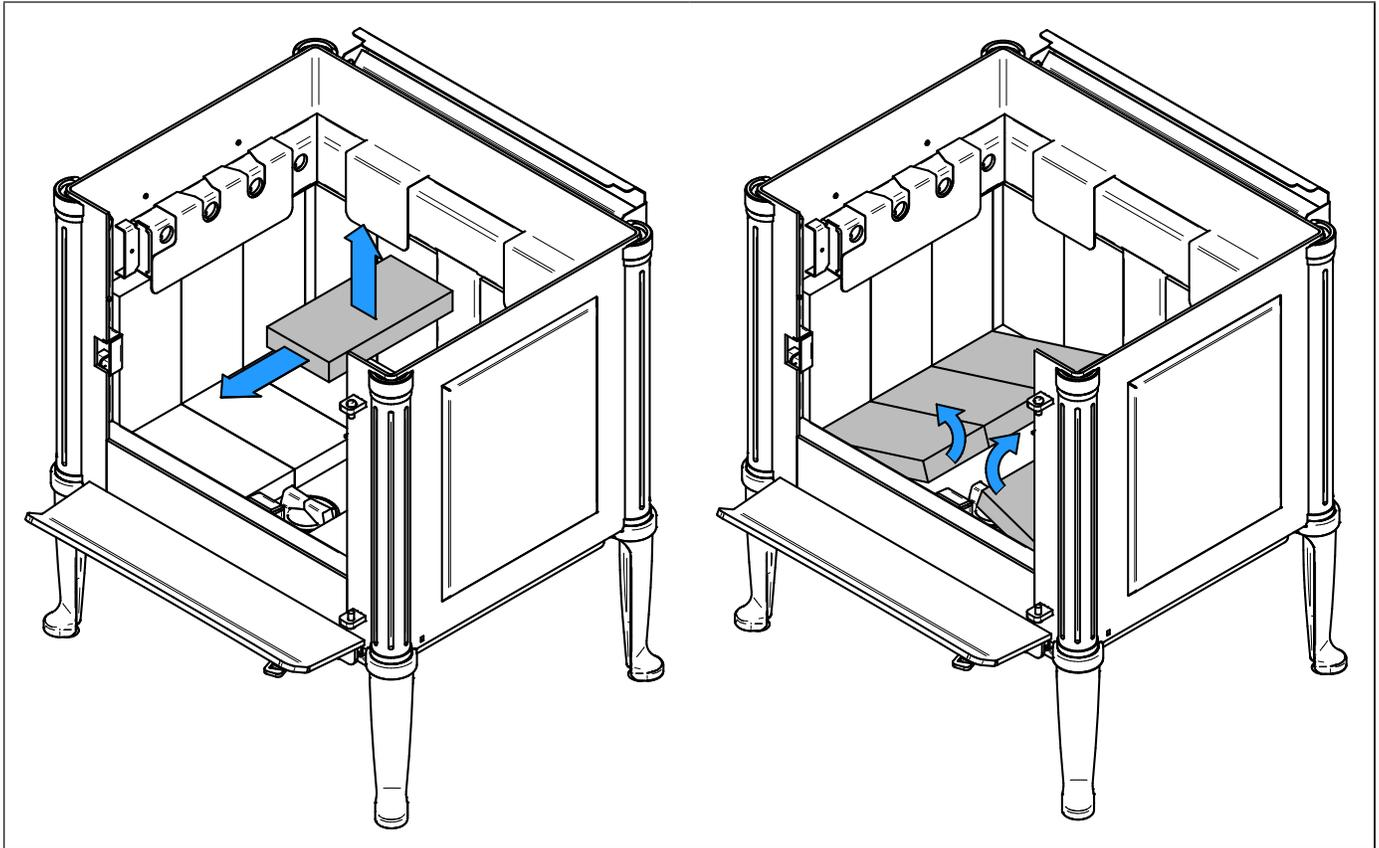
1. Remove the center floor brick and then remove the 6 other floor bricks.
