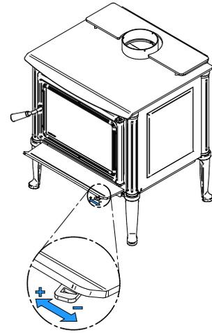
Figure 9: Air Intake Control
