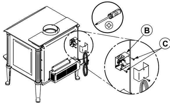
2. Screw the blower **(E)** in place using the screws **(D)** included in the installation manual. Screw the thermodisc **(B)** with the screws **(C)** supplied with the thermodisc on the back of the stove.
