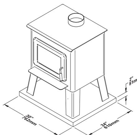
Figure 18: Floor protection in a mobile home
