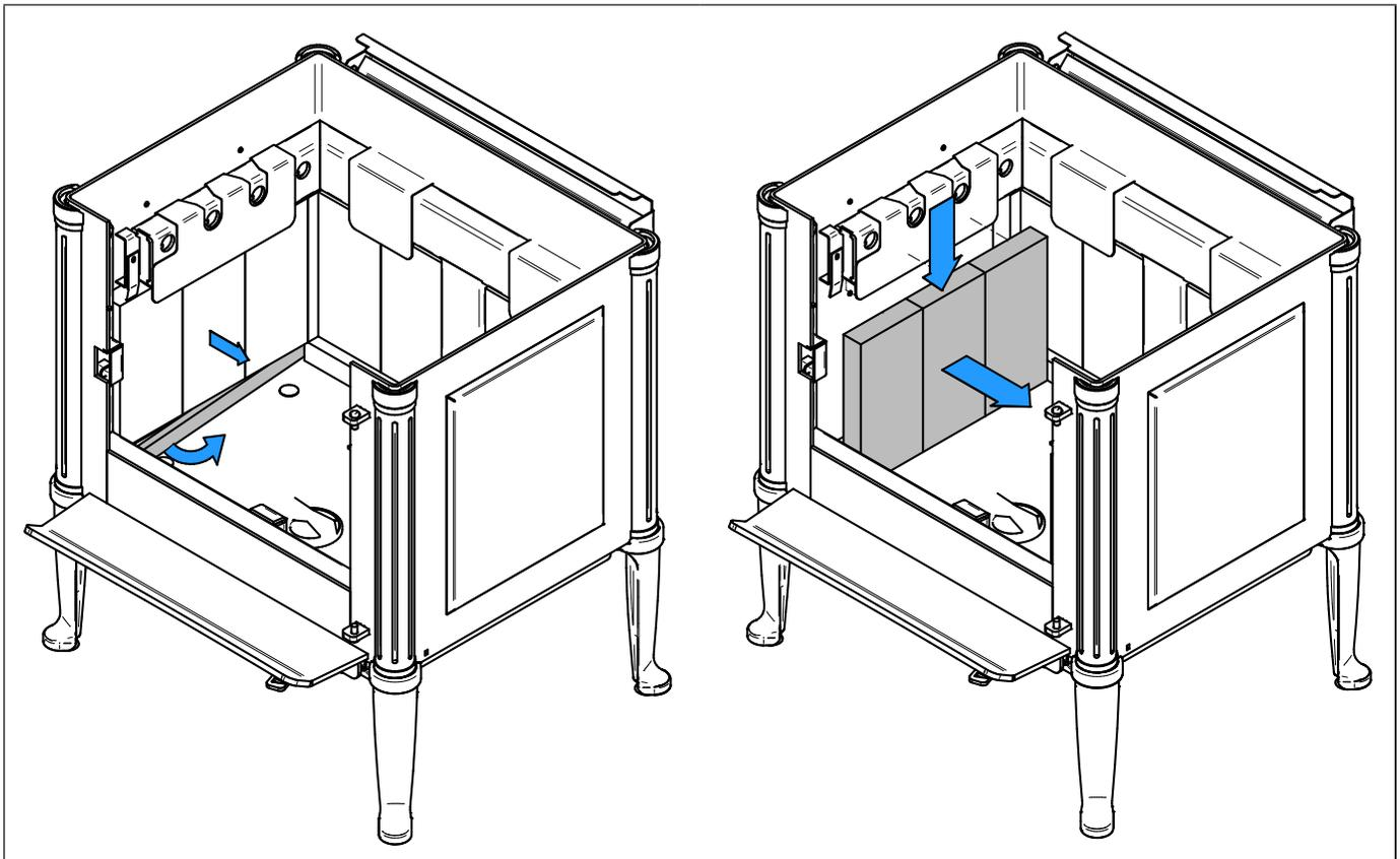
2. Remove the brick holder and remove the three left side bricks. Redo for the right side.
