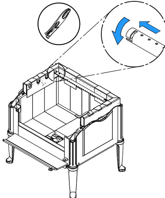
2. Align the notch in the left end of the tube with the key of the left air channel hole. Using a « Wise grip » hold the tube and lock it in place by turning the tube as shown. Make sure the notch reaches the end of the key way.
