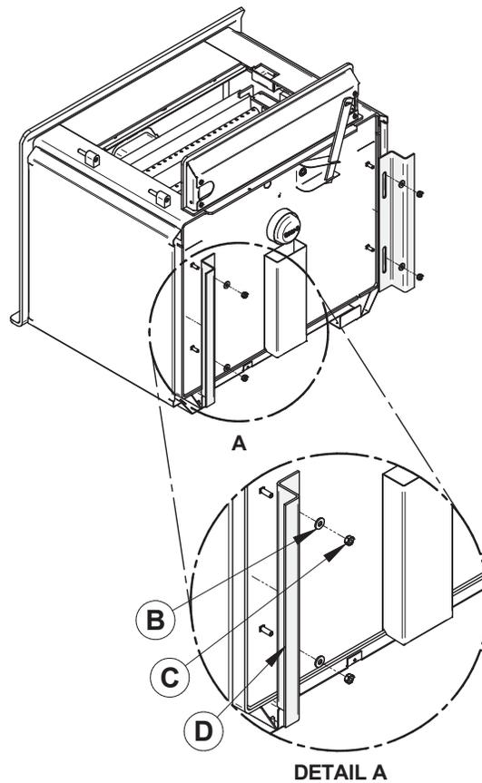
2. Put the stove on its back. Remove and dispose of the two freight supports **(D)**. Keep the nuts **(C)** and washers **(B)** for step 3.
