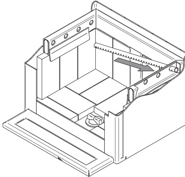
1. Starting with the rear tube, lean and shove the right end of the secondary air tube into the rear right channel hole. Then lift and shove the left end of the tube into the rear left channel.
