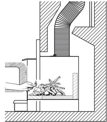
**DO NOT LEAVE THE STOVE UNATTENDED WHEN THE DOOR IS SLIGHTLY OPENED. ALWAYS CLOSE AND LATCH THE DOOR AFTER THE FIRE IGNITES.**
