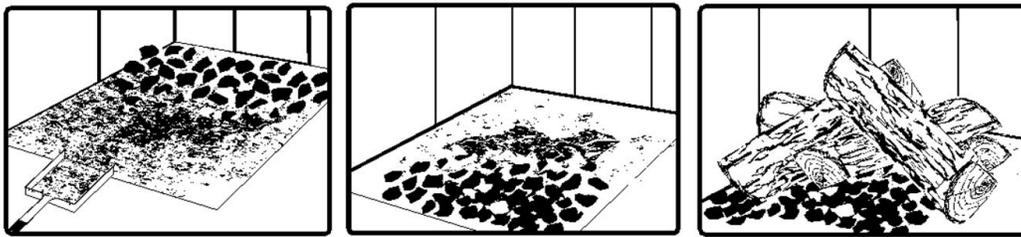
Remove ash first, and then rake charcoal towards the front of the firebox before loading so that it will ignite the new load.
