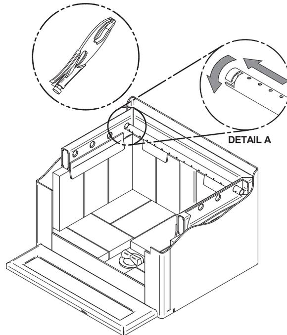
2. Align the notch in the left end of the tube with the key of the left air channel hole. Using a « Wise grip » hold the tube and lock it in place by turning the tube as shown in detail A . Make sure the notch reaches the end of the key way.
