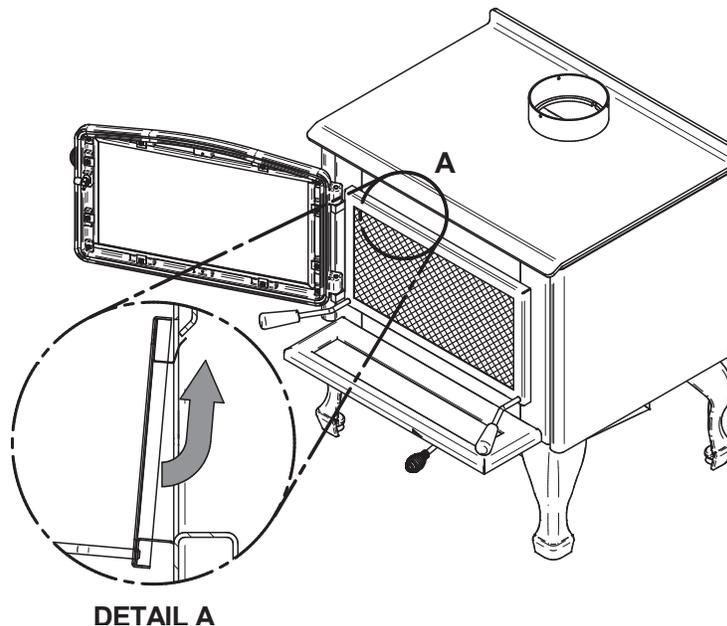
3. Lean the upper part of the fire screen against the top door opening making sure to shove the top fire screen brackets behind the primary air deflector.
