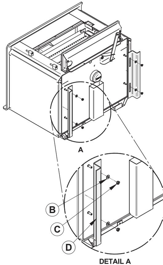
2. Put the stove on its back. Remove and dispose of the two freight supports **(D)**. Keep the nuts **(C)** and washers **(B)** for step 4.
